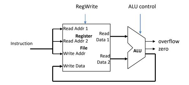
Note that Register File is not written every cycle (e.g., **sw**), so we need an explicit write control signal for the Register File
